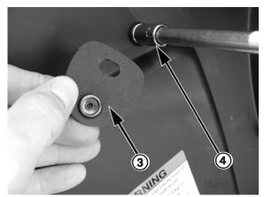
Install two of the mounting tabs (preferably the bottom two as the lid is oriented when it is open) to the rack's studs. Put the washer ⑤ on the outside of the tab and then hand-install the nut.
