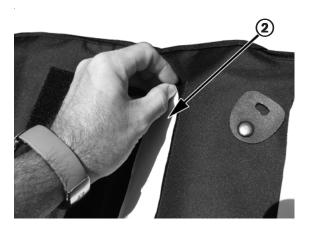
Position the organizer ③ to where you desire it to be placed in the lid and press down firmly so the adhesive backing of the strips stick well to the inner trunk lid.
