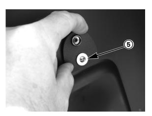
Connect the organizer's two bottom snaps to the mounting tabs snaps. You may need to rotate or adjust the position of the tabs for the snap align with the snaps on the back of the organizer. Once the tabs and the organizer snaps are firmly connected, tighten the rack's nuts to the torque specified by the rack's manufacturer.
