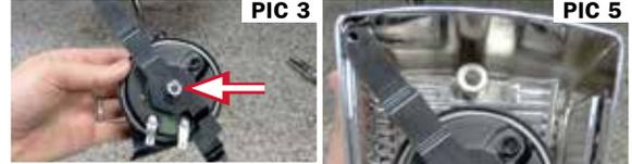
**STEP 6** Refer to PIC 5. Place the horn and bracket assembly inside of the horn cover, with the longer arm in the upper left corner and shorter arm in the lower right corner. Adjust the position of the horn to be sure the terminal connect points of the horn are pointing down towards the ground. Fully tighten the flange nut to secure the horn in place.
