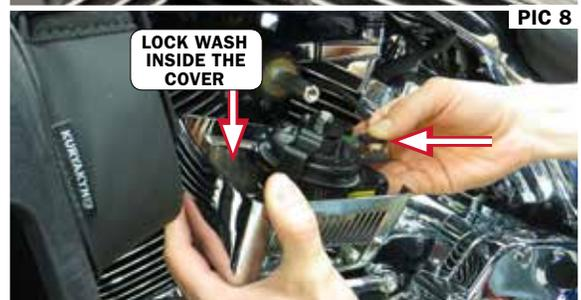
**STEP 10** Refer to PIC 8. Reattach the horn wires to the terminal connect points on the horn.
