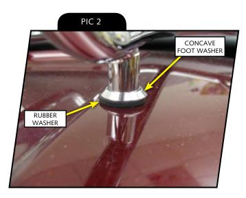
**STEP 6** To mount the rear portion of the luggage rack, remove the masking tape from the two rear holes. Using the same operation from the previous step, mount the rear portion of the rack. Tighten both the front and the rear bolts of the luggage rack. (Be sure not to over tighten the screws, damage to the lid will occur)
