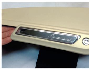
5. Carefully position Saddlebag Hinge Insert in place, press to adhere.
