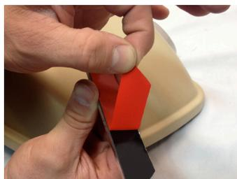
4. Remove backing from the Saddlebag Hinge Insert.
