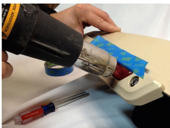
1. Carefully release the bond and start removal of stock reflector.
