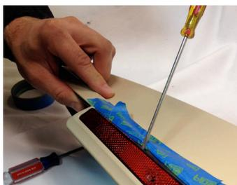
2. Gently lift reflector off stock saddlebag latch once adhesive bond is released.
