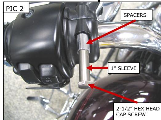
**MOUNT OPTION 2: Mounting to clutch or brake perch.**
