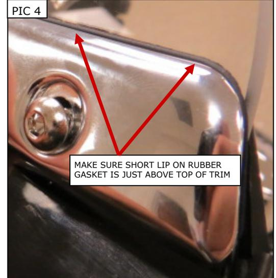
**NOTICE** It is the installer's responsibility to ensure that all of the fasteners (including pre-assembled) are tightened before operation of the motorcycle. Küryakyn will not provide warranty coverage on products or components lost due to improper installation or lack of maintenance. Periodic inspection and maintenance are required on all fasteners.
