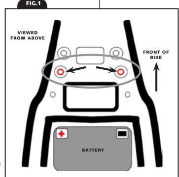
**STEP 5** Remove any grease or debris from the installation area (See <u>FIG.1</u> and <u>PIC.1</u>) with soapy water and a clean rag; allow the area to dry completely.
