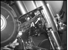
Step #9: The balance of the main wire harness will pass through on the brake side of the fairing where the main factory wires pass as shown by "A" in the image. Have the opposite end of the main harness go so it ends up on top of the crash bar as close to the center as you can.
