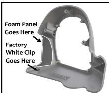
Step #6: The kit comes with die cut foam panels. Find the one for the side of the bike you are working on and apply as shown noting you should clean the area with isopropyl alcohol first. On your factory front panel, you will see 2 white clips. One of these clips will come off and be installed onto the Hogtunes main panel.
