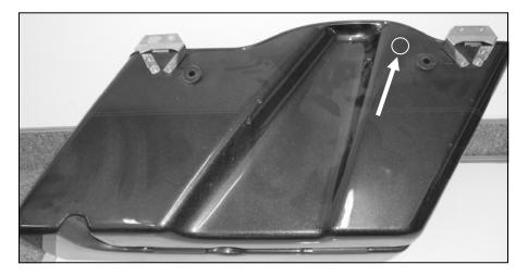
The white circle in the picture above is where a 3/4" (19mm) hole will be drilled. This hole is where the supplied Hogtunes rubber grommet will go, and allow the speaker wire for the lid to pass into the saddlebag. Note: We strongly suggest putting masking tape over the area to be drilled before making the hole. We also strongly suggest starting with a small bit, and gradually working your way up to the 3/4" (19mm) hole.
