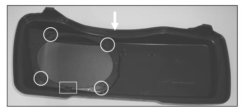
With the gasket installed, you will insert the factory metal strip (5 screws) between the gasket and new lid. Re-install the 5 factory machine screws the same way they came off the factory lid. The new lid will now be at-tached to your saddlebag.
