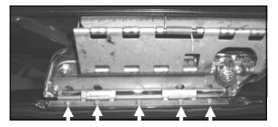
With the flap off, fold the factory lid all the way over, exposing the 5 screws highlighted above by white arrows. When these are removed, the factory lid will be free from the saddlebag. These screws will be used to install the new lid so keep them handy.
