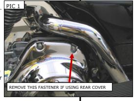
STEP 5 Install the included 1/4"-20 x 5" socket head cap screw in the front hole on the cover. Install the included 1/4"-20 x 1-1/2" socket head cap screws in the next two holes. Place an aluminum locating washer over the protruding end of each 1/4"-20 fastener; ensure that the round side of the washer is facing toward the hole in the primary chain case. FIG 1
