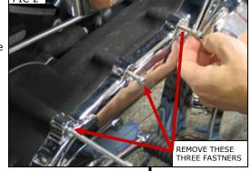
Position the cover assembly in place. Slide the rear section of the cover assembly into place and then pivot the front section into place. Be patient, this may take some finesse. Tighten the #10-24 fastener at this time.
