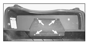
Remove the 4 screws (highlighted with white arrows above) that hold the cloth flap in place. With the flap off, slide one of the metal bars out from inside the flap as it will be used for new lid. The screws just removed will be
