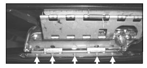
With the flap off, fold the factory lid all the way over, exposing the 5 screws highlighted above by white arrows. When these are removed, the factory lid will be free from the saddlebag. These screws will be used to install the new lid so keep them handy. With the factory lid off the bike, you will see a metal "strip" between the rubber gasket and the lid itself that the screws just removed threaded into. This metal strip must be removed as it will be used to install the new lid.
