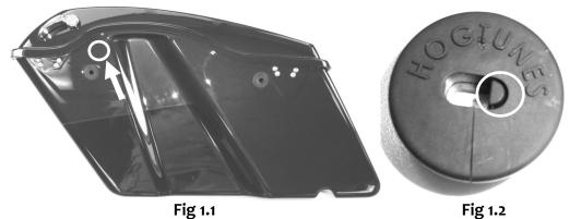
The white circle in Fig 1.1 above is where a 3/4" (19mm) hole will be drilled. This hole is where the supplied Hogtunes rubber grommet will go, and allow the lids speaker wire to pass from the saddlebag. We strongly suggest putting masking tape over the painted area to be drilled. We also suggest starting with a small bit, and gradually working your way up to the 3/4" (19mm) hole. Drilling the hole with the lid still on is a good idea!!
