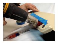
Carefully release the bond and start removal of stock reflector.
