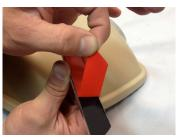
**4.** Remove backing from the Saddlebag Hinge Insert.
