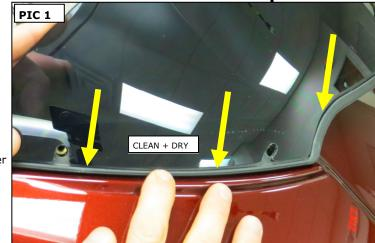
**STEP 5** Ensure that the windshield rests on the existing rubber seal as shown in **PIC 1.**
