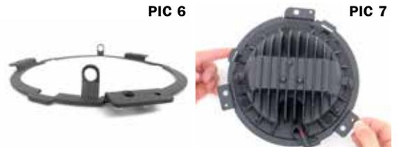
**STEP 6** Refer to PIC 8. Align the two inner brackets of the Headlight Mounting Bracket with the holes on each side of the Headlight. Fasten the Mounting Bracket to the Headlight by placing a 8MM split washer on each of the M8 screws and inserting them through the aligned side holes, one on each side. Fully tighten hardware.
