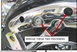
WARNING BOTH PIVOT/HINGE SCREWS MUST HAVE THREADLOCK COMPOUND RE-APPLIED AND RE-TORQUED ONCE REMOVED
